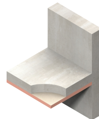
Insulation for structural ceilings (soffits)
